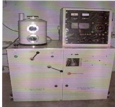
Figure 4: HINDHIVAC Vacuum Coater
